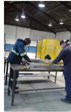
Busy making safety gates
